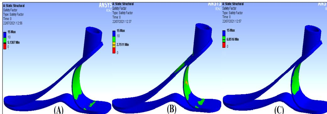
Figure 18. (a) The safety factor value for carbon fiber reinforced foot model at the heel strike stage; (b) The safety factor value for fiberglass reinforced foot model at the heel strike stage; (c) The safety factor value for hybrid material reinforced foot model at the midstance stage
